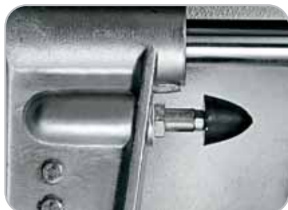
Paracolpo carrello Hopper's buffer
